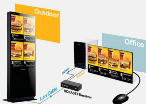
Figure 8. Remote management of outdoor signage with simple, low-cost connection through advanced HDBaseT
